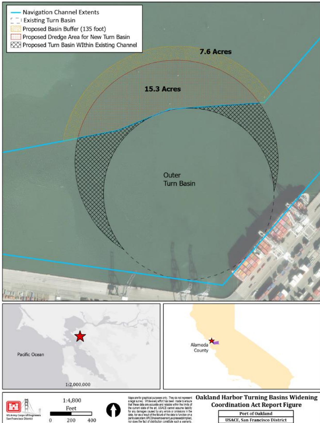
Figure 2. Outer Harbor Turning Basin widening footprint.
